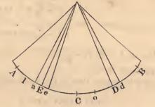
COR. The greatest velocity in a resisting medium is at the point o.
